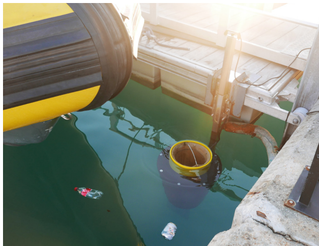
Sea bin in the water after installation
