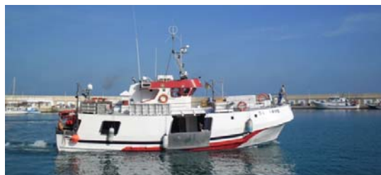
Figure 47. A large Spanish bottom longliner, from Port of Carboneras.
