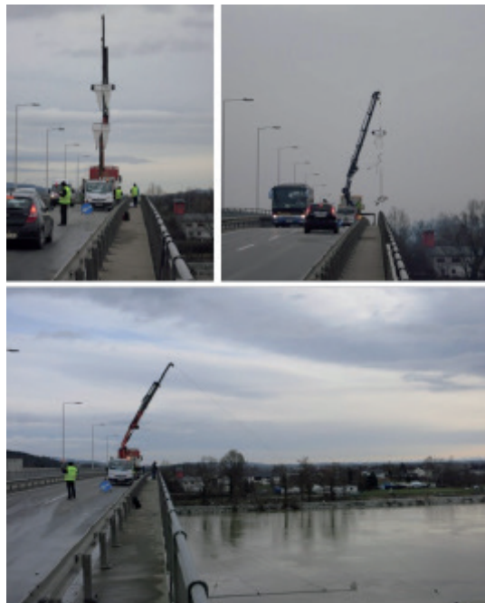
Figure 3. Sampling a large river (the Danube) by crane from a bridge. An array of nets is positioned to sample the water surface and the water columns simultaneously (Hohenblum et al. 2015).
