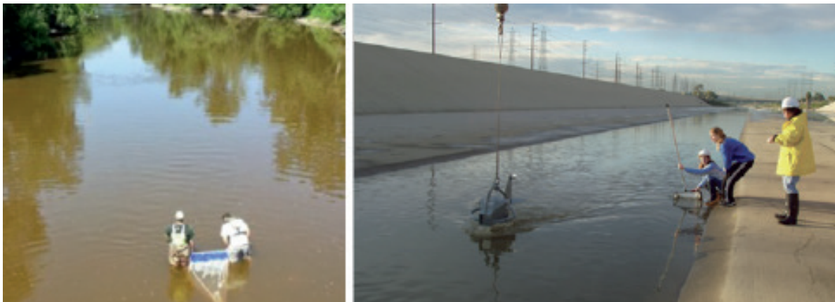
Figure 2. Examples of the use of sampling nets in a wadable river (left, Baldwin et al. 2016) and from the bank and a crane (right, Moore, Lattin and Zellers 2011)
