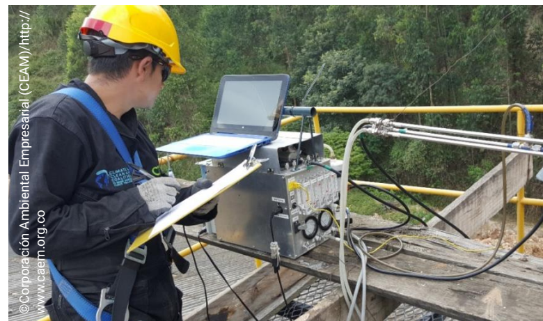
Black carbon measurements taken at a brick kiln in Colombia
