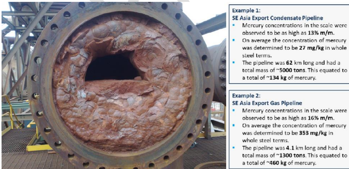
581 Figure 5. Solid waste accumulated on the inner surface of a pipeline (left) and 582 case studies (right). Data provided by Qa3.
