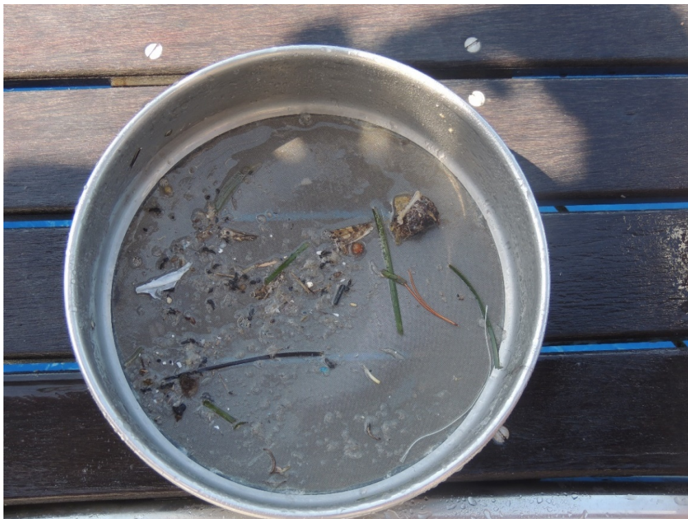
Figure 3: Microplastic and organic matter collected in a metal sieve just after the sampling (Photo: © Christos Ioakeimidis, UNEP/MAP).
