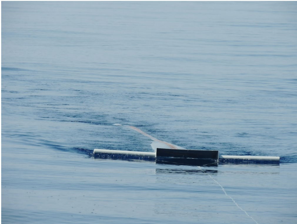
Figure 1: Manta net being operated in calm sea, outside of the bow wave caused by the spinning of the propeller (Photo: © Christos Ioakeimidis, UNEP/MAP).
