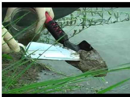
Figure 5. Hand-held scoop sediment sampler
