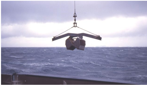
Large grab sampler (picture: S. de Mora)
