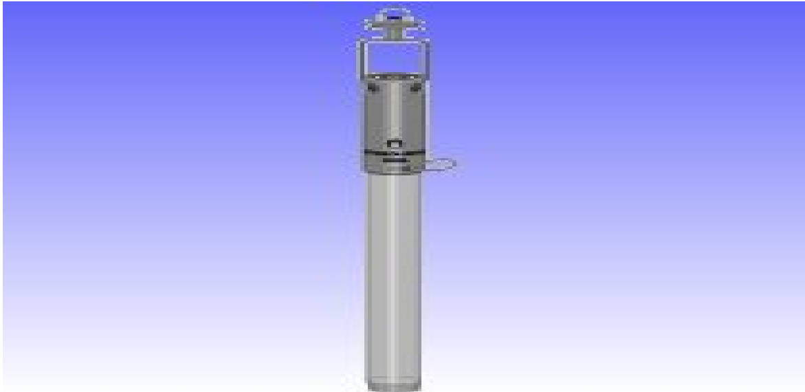
Figure 3: Gravity corer (picture from Hydro-Bios, Germany).
