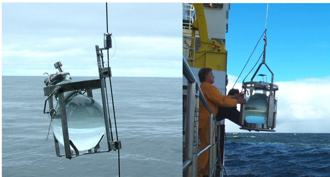
Figure 3 Left: BSH all-glass bottle water sampler (10 l). Right: 100 l glass flask sampler for sampling seawater for the analysis of organic contaminants.
