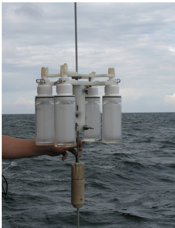
Figure 2 Modified MERCOS water sampler of the second generation for four bottles, manufactured by BSH, Germany (photo courtesy of S. Schmolke, BSH, Germany).
