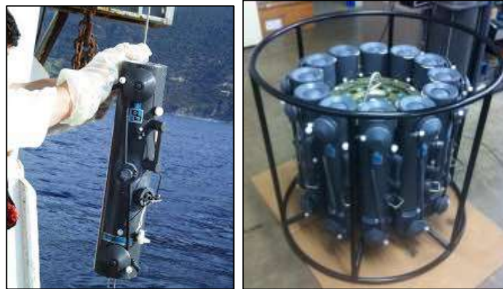
Figure 1. Individual GO FLO seawater sampler and rosette system with multiple samplers
