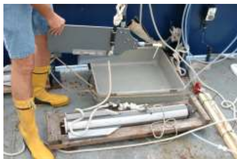
Figure 3. Surface pump sipper/tow fish system (GEOTRACES, 2017)
