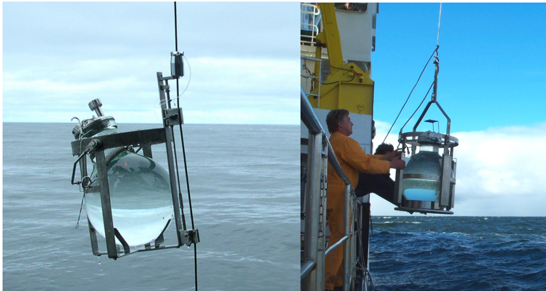
Figure 3 Left: BSH all-glass bottle water sampler (10 l). Right: 100 l glass flask sampler for sampling seawater for the analysis of organic contaminants.
