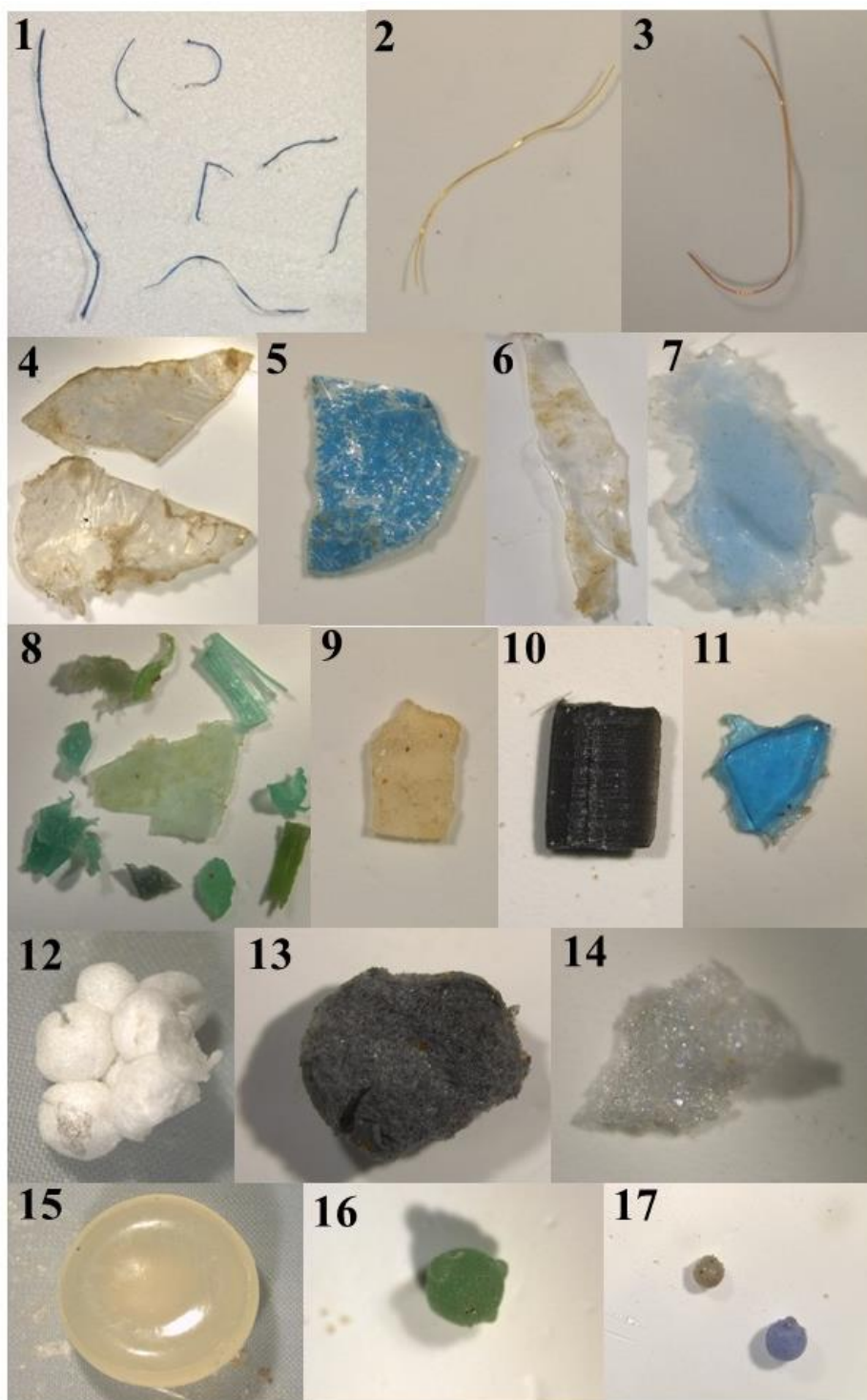
Figure 4: Common shapes of microplastics. (1: fibers, 2-3: filaments, 4-7: films, 8-11: fragments, 12-14: foams, 15: pellet, 16-17: granule) (Photo: © Ülgen Aytan, Turkey).
