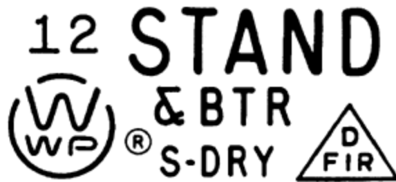
Figure 1. Example of grade mark, with mill identification, grade designation, species, seasoning and moisture content. It can also include a trademark.
