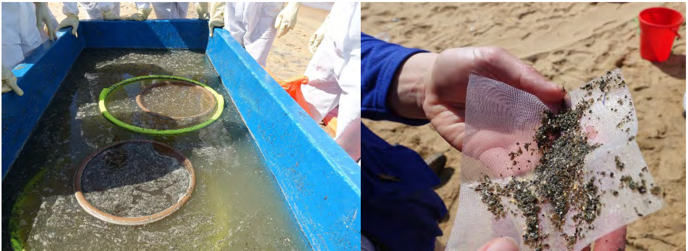
Figure 2.23: Burnt plastic particles left after flotation that are too small to be recovered with existing sieves.
