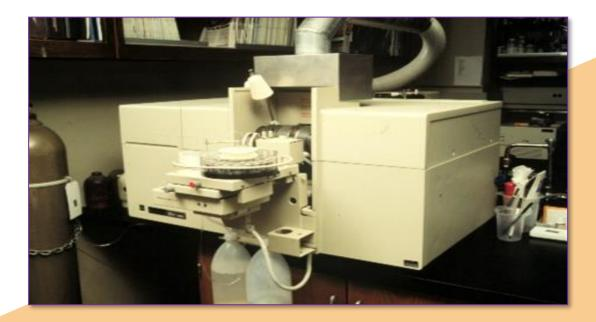
Method 3: Inductively Coupled Plasma Atomic Emission Spectrometry (ICP-AES)
