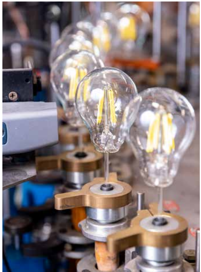
Automated workshop conveyor for production of glass lamps bulbs factory. © Parilov/Shutterstock.com.
