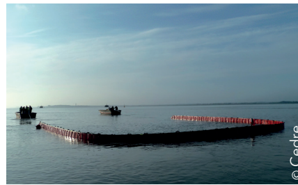
Dynamic containment with conventional inflatable booms in a "U" configuration
