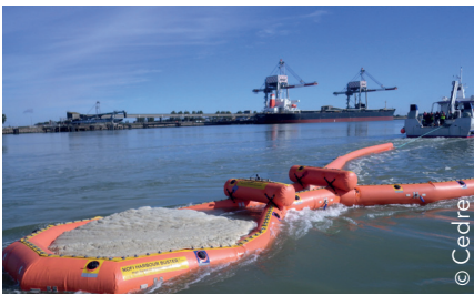
Dynamic containment with a Current Buster
