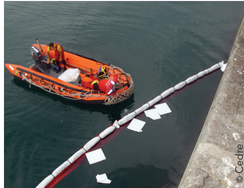
Sorbent sheets are applied to recover floating liquid pollutant with low/medium viscosity
