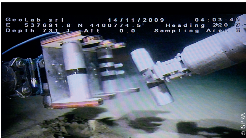
Sediment sampling with a ROV on the deep seafloor
