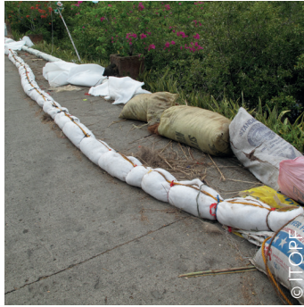
Custom-made boom made with hay
