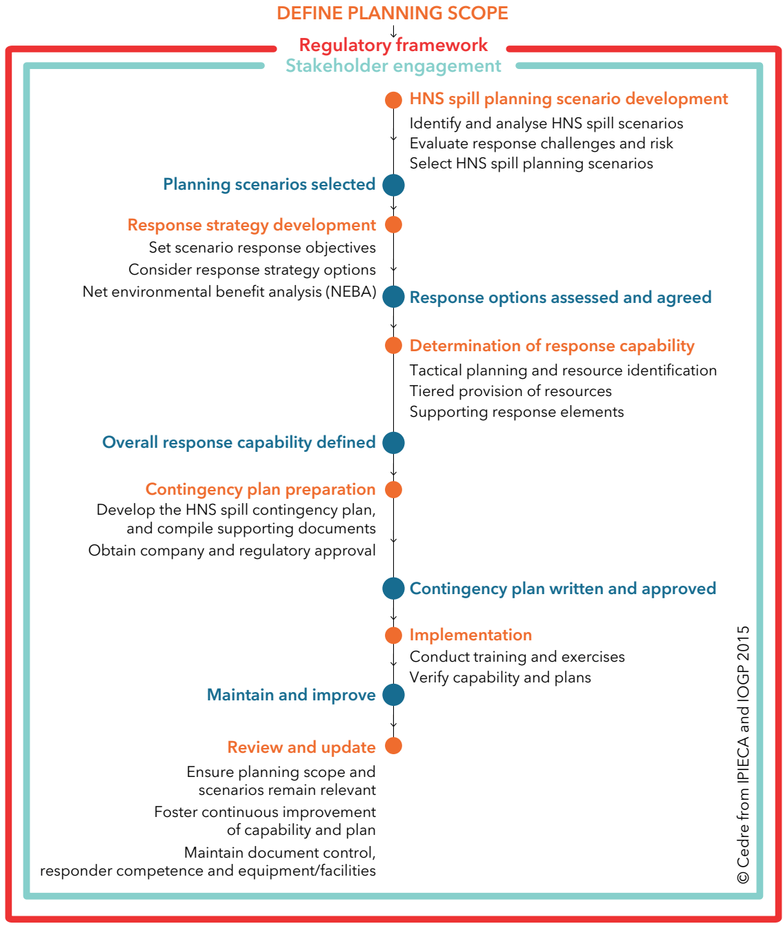
Figure 22: The overall process for industrial contingency planning
