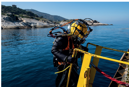
Diver equipped with a rigid helmet and a vulcanised dry suit
