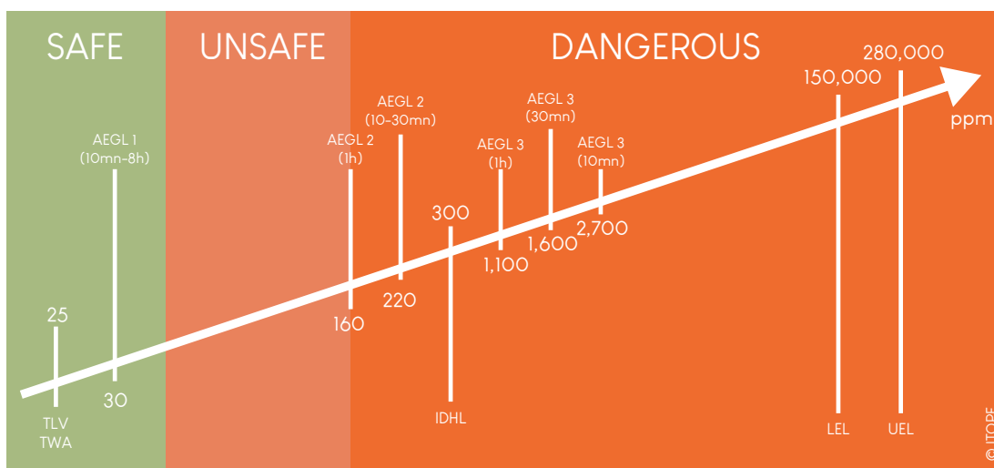
Figure 15: Representation of flammability and inhalation hazards of ammonia for responders
