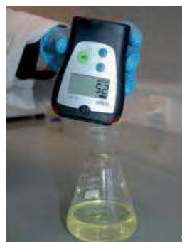
Vapour measurement with an explosimeter
