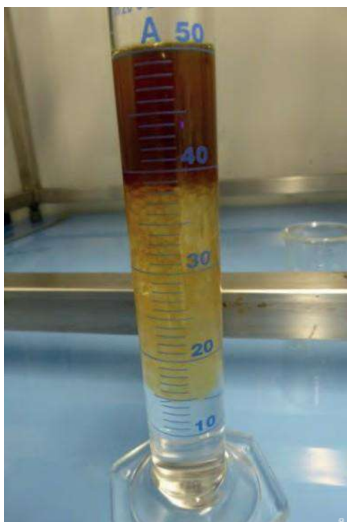
Rapid settling of the Vega condensate in the absence of agitation
