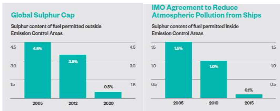
Figure 117. Global Sulphur Cap – IMO Agreement to reduce atmospheric pollution from ships. Source: International Chamber of Shipping, 2019 [16]
