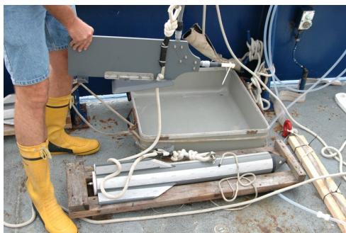
Figure 3. Surface pump sipper/tow fish system (GEOTRACES, 2017)
