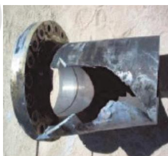
Figure 5: Metallurgical failure caused by mercury in a gas processing facility (IPIECA).
