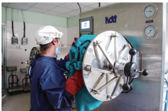
Figure 15: Waste autoclaves in operation (left), and monitoring (right) (Source: HECAF 360)
