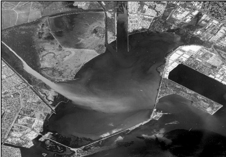
Figure 22. Typical behavior of the suspended solids “jet” from Río Cobre in Hunts Bay, Kingston Harbour, Jamaica
