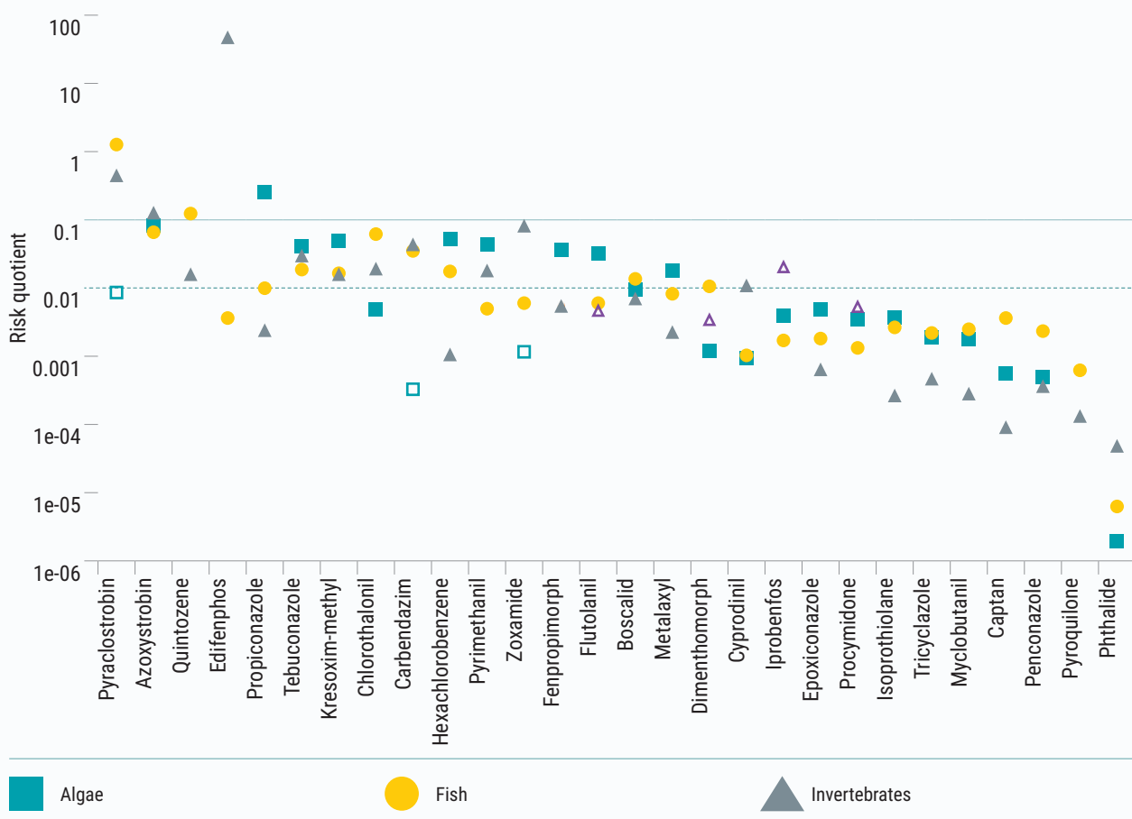
▶ Figure 4.3.5-1 Risk quotients for algae (squares), fish (circles) and invertebrates (triangles) as ratios of maximum detected global field concentrations and acute standard toxicity data. Open symbols indicate that toxicity was provided as “greater than” values. Risk quotients > 0.01 (dashed line) and > 0.1 (solid line) indicate moderate and high risks, respectively. Zubrod et al. (2019).
