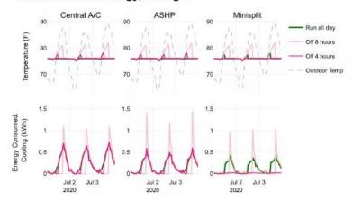
The researchers used the same three different HVAC technologies and three temperature-setting strategies, but this time for a house in hot and found Atlanta. Pigott/Scheib/Baker/CU Boulder, CC BY-ND
