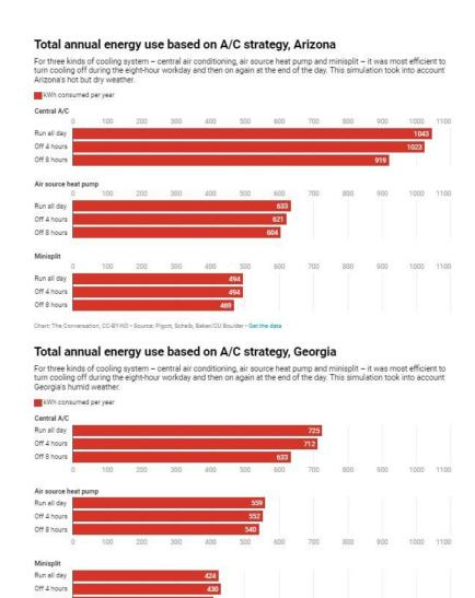
The central air source heat pump and minisplit heat pump are more efficient overall but yield less savings from temperature setbacks. An eight-hour setback on weekdays provides savings regardless of the system type, while the benefits gleaned from a four-hour setback are less straightforward.
