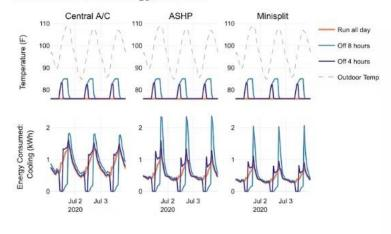
Energy models can show how much energy a house will use under particular conditions – like Phoenix's hot, dry summer weather. The researchers ran the numbers on three different HVAC technologies and three different temperature-setting strategies. PigotiScheib/Baker/CU Boulder, CC BY-ND
