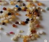
Industrial plastic granules, usually cylindrical but also sometimes oval spherical or cubical shapes, or suspected industrial item, used for the tiny spheres (e.g., glassy, milky etc.) |
