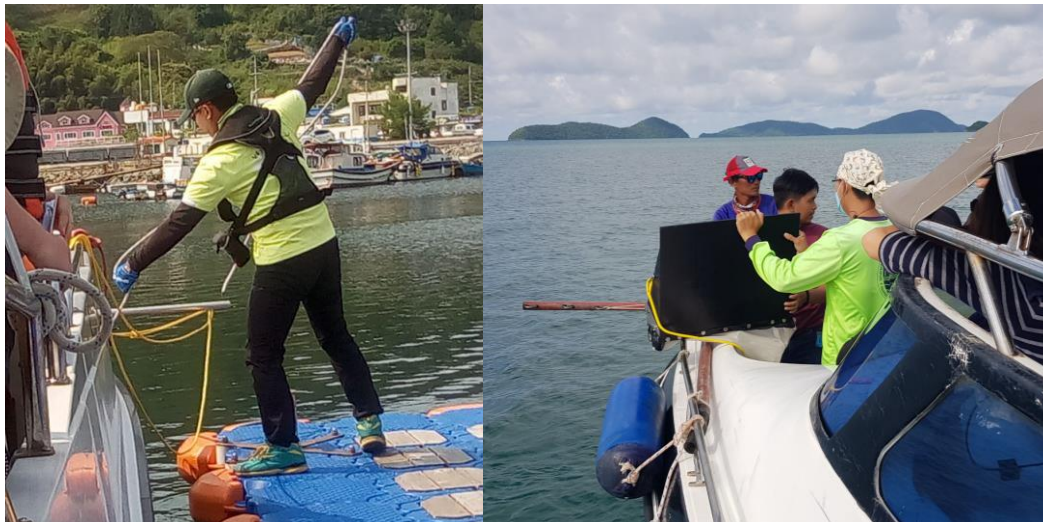
Figure 14: Examples of booms on the side of boats for attaching the trawl net via the tow rope.
