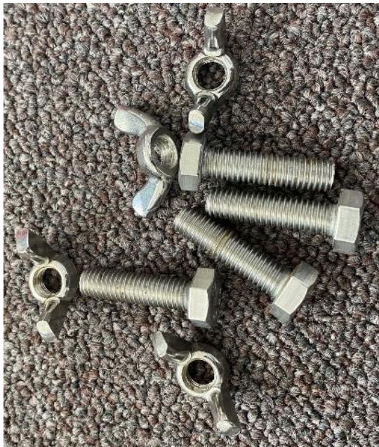
Screws and wingnuts to hold the sides of the frame
