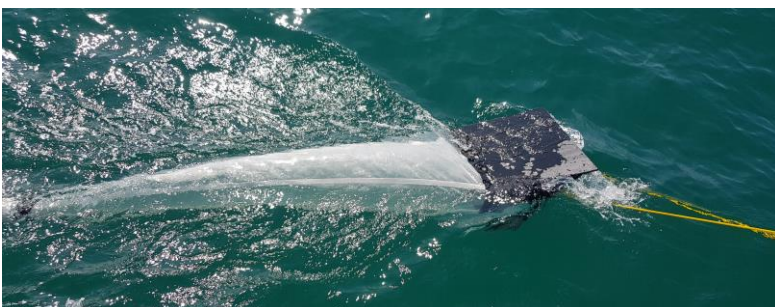
Figure 15: The large black square panel is on the top side of the net when sampling.
