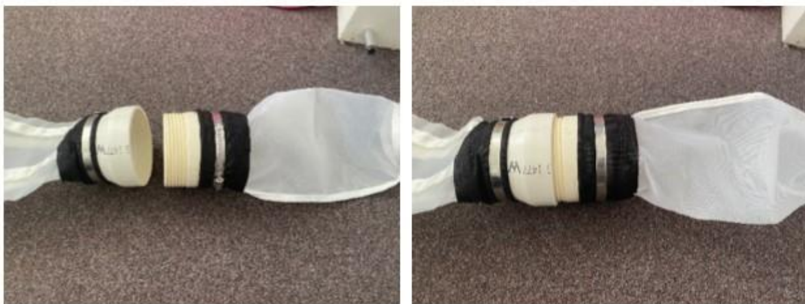
Screw the cod end onto the net
