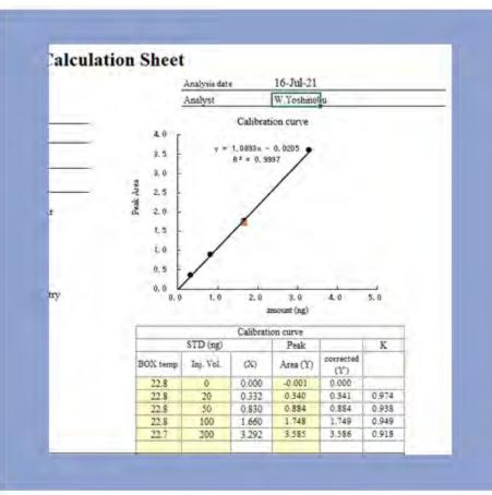
Make the standards for calibration curve by converting the saturated gaseous mercury added
