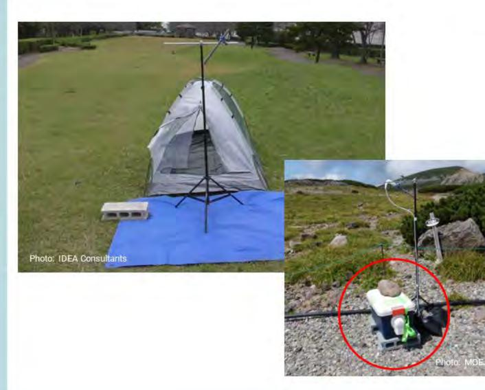
If the ground is bare soil, or with a lot of dust, covering with a sheet is desirable.
