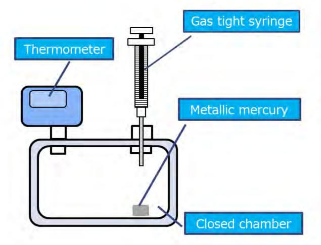
Draw saturated gaseous mercury from closed chamber containing metallic mercury
