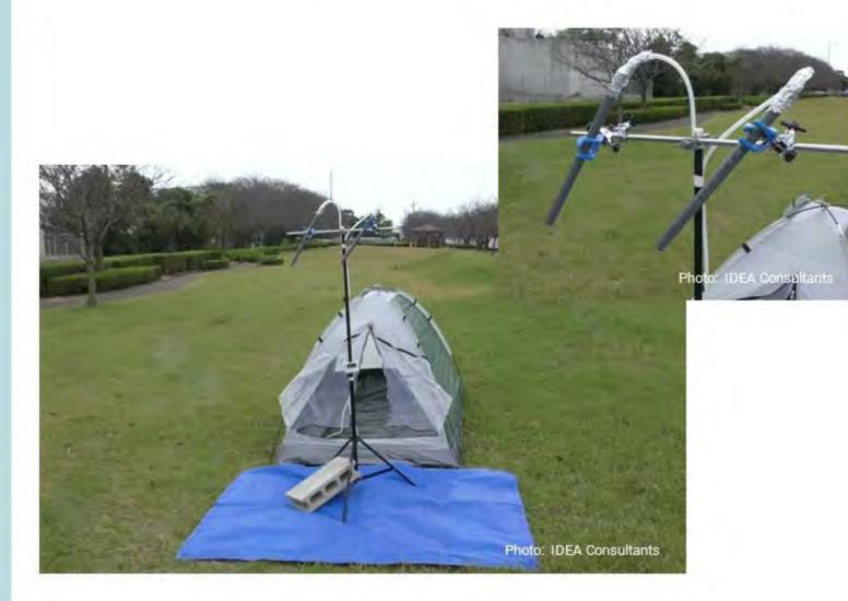
□To confirm the stability (precision) of the survey, 1 pair of duplicate sampling on 10 samplings is recommended. Deploy 2 (or more) cartridges side by side.
