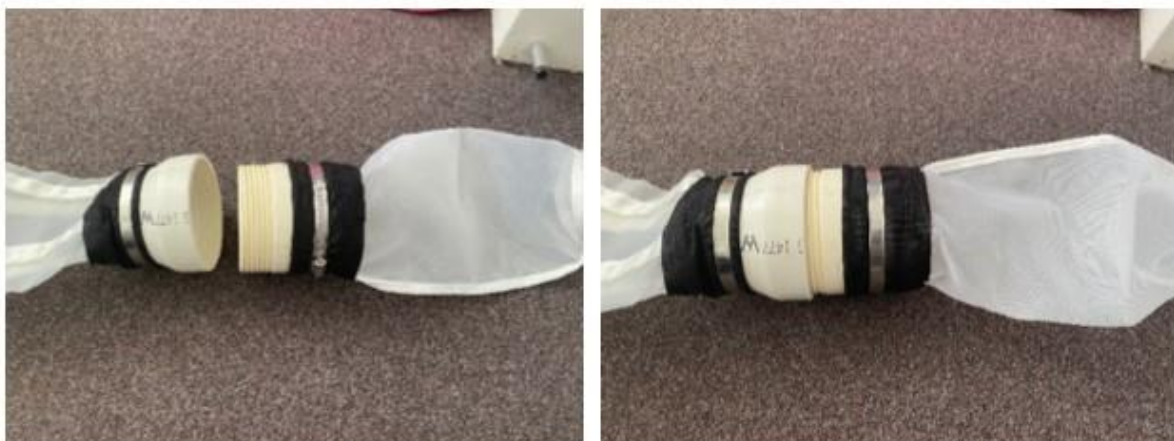
Screw the cod end onto the net
