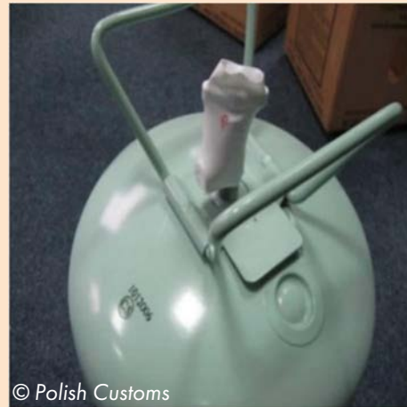
Photo 3.45 Typical non-refillable cylinders 4
