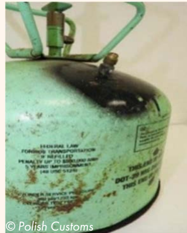
Photo 3.51 Altered non-refillable cylinder
