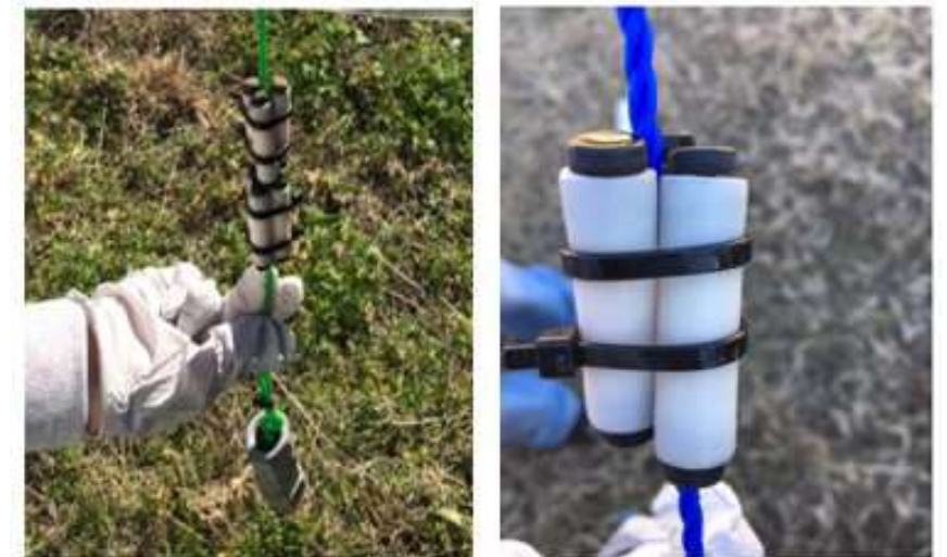
PFAS passive water samplers
