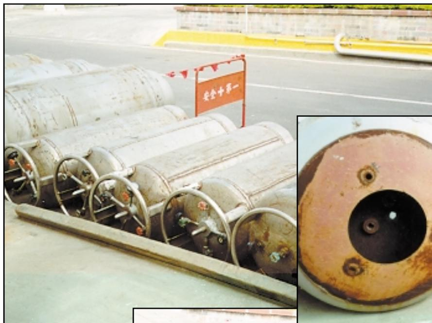
Seized refrigerant containers with a hidden compartment containing CFC-12. Access valves were connected to a small compartment containing HFC-134a.
