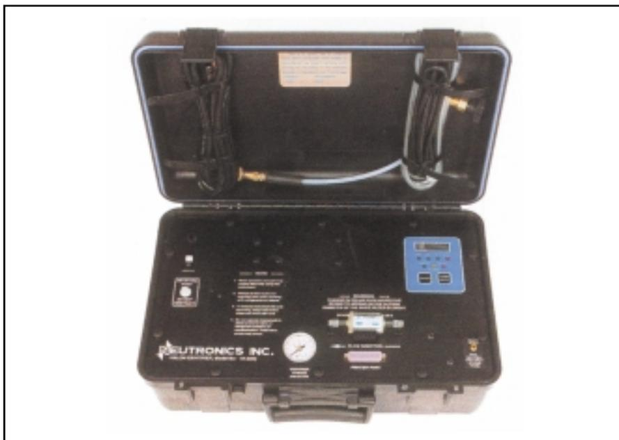
A portable Halon Identifier used to analyse liquid samples to verify purity and identify contaminants taken from storage cylinders.
