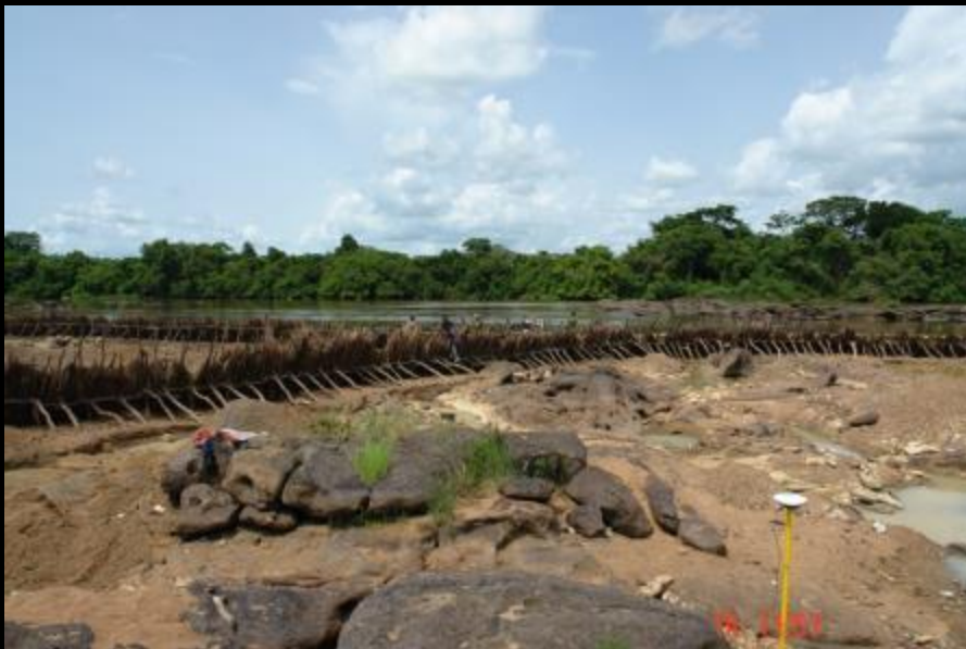
Image Credit: Pete Chirico, USGS Barrage diamond mining site at Bada/Touya, Central African Republic - May, 2007
