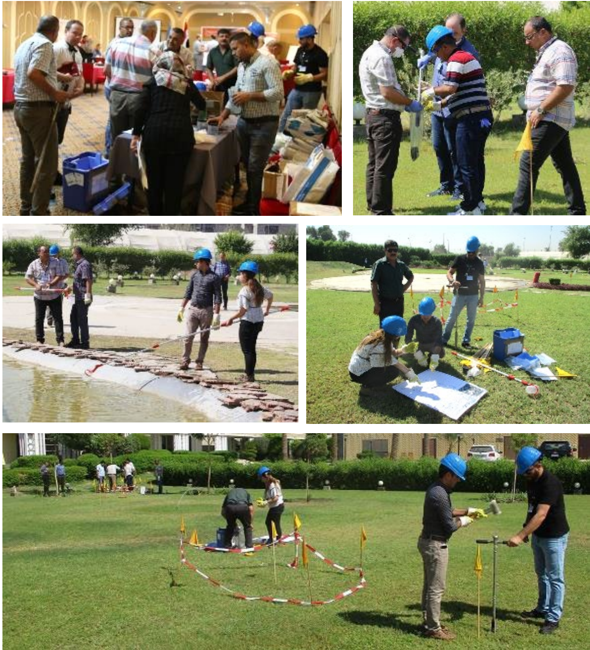
Figure 5: The five assessment teams prepare their field sampling kits (top left), and in the garden of the Al Rasheed Hotel conduct Detailed Site Assessment work with collection of water and soil samples from each contaminated scenario site based on the Conceptual Site Model they previously prepared.
