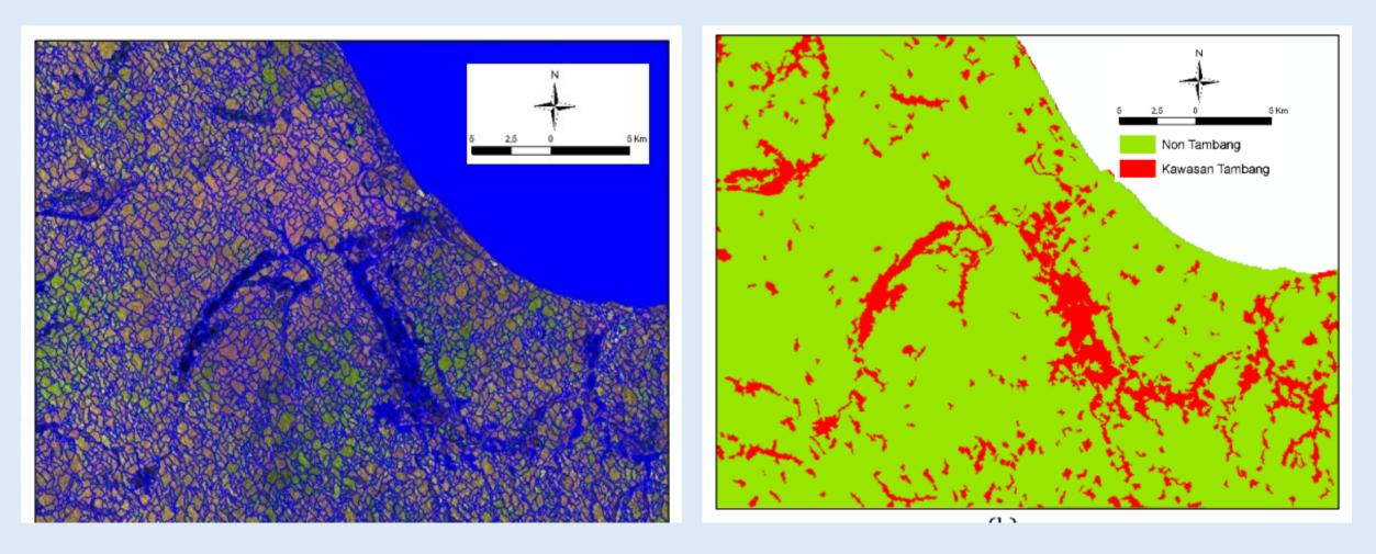
Open mining detection with Object Based Image Analysis (OBIA) with texture approach from Sentinel – 1 (radar data). This work support local government to analysis the environment impact.
