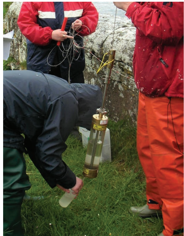
Figure 3.2 Filling a sample bottle from a Ruttner grab sampler. Neither the sampler nor the bottle must touch the ground until the bottle is filled and the lid is tightly closed. © Deborah Chapman
