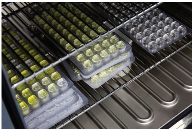
Figure 8.4 An example of a commercially available multiple well assay tray for E. coli © Jean O'Dwyer
