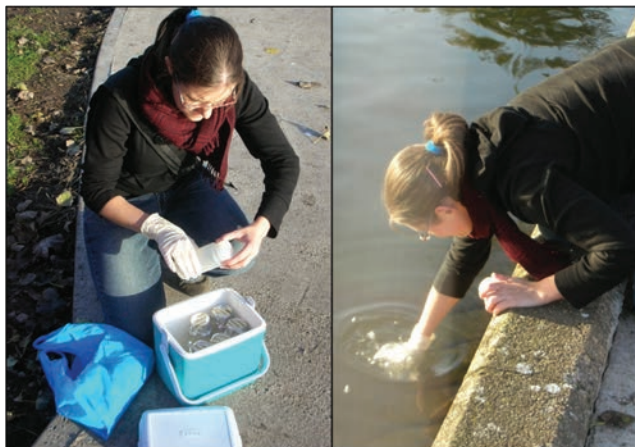
Figure 3.3 Taking a grab sample directly into the sample container. © Deborah Chapman
