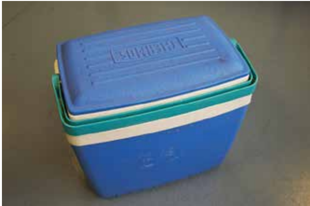
Figure 6.1 Example of a coolbox for transporting samples back to the laboratory © Patrick Cross
