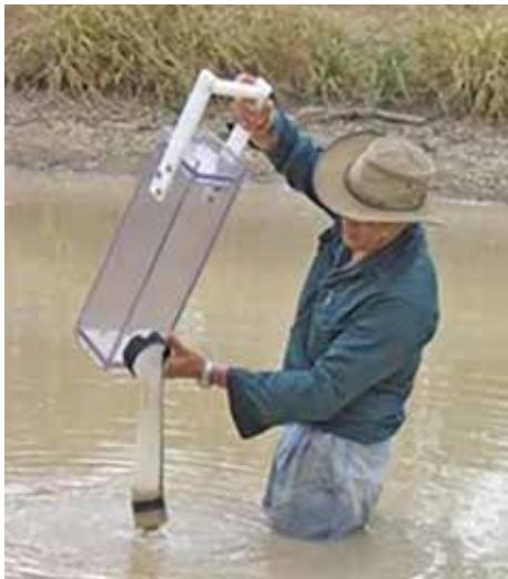
Figure 6.12 Collecting a plankton sample with a Schindler-Patalas trap (DES 2018) By State of Queensland, Licenced under CC BY 3.0 AU
