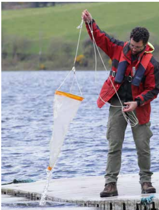
Figure 6.13 Sampling the water column for plankton by taking a vertical haul with a plankton net © Patrick Cross
