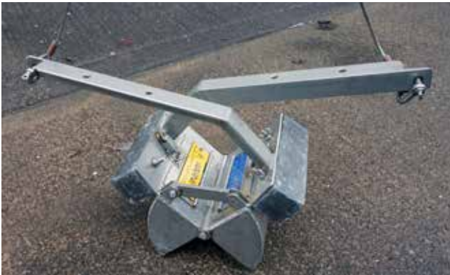
Figure 6.10 A Van Veen grab for collecting sediment samples © Patrick Cross
