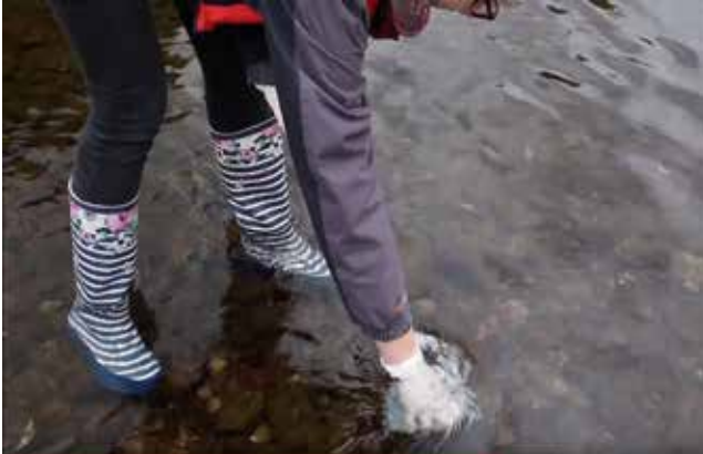
Figure 6.3 Taking a dip sample directly from the water body using the sample bottle © Patrick Cross
