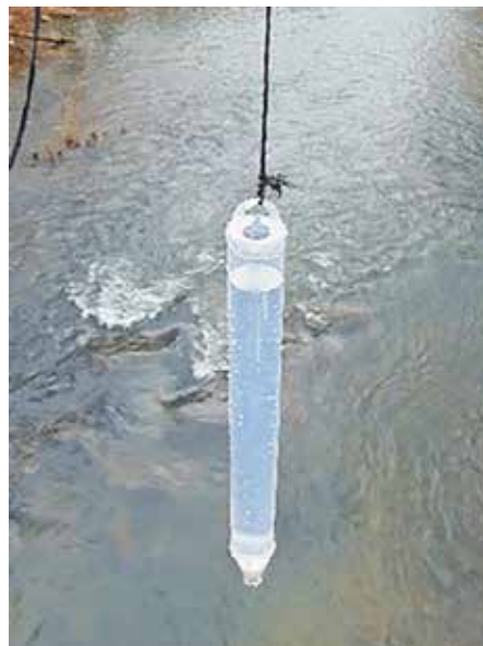
Figure 6.6 Teflon® bailer used for water sample collection (Kaur et al. 2018). Licensed under CC BY 4.0
