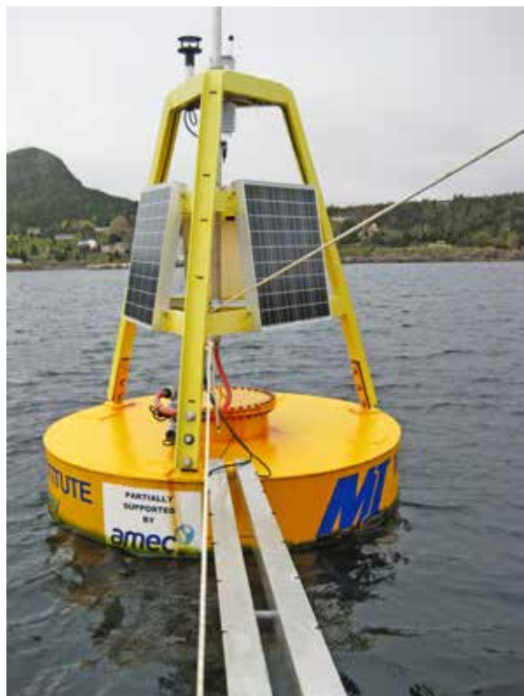
Figure 6.15 An anchored buoy with continuous monitoring sensors suspended at depth underneath. Solar panels provide power for the sensors and telemetry system. © Timothy Sullivan
