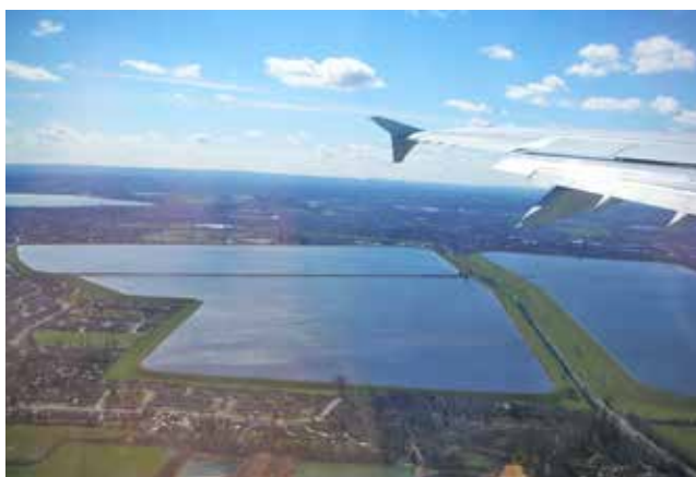
Figure 4.3 Embanked reservoirs built to supply drinking water to London. © Deborah Chapman
