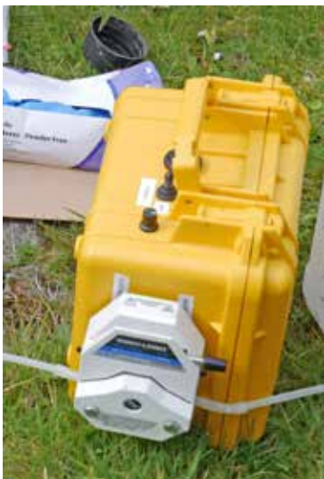
Figure 6.7 A portable peristaltic pump that can be used to take samples from depth in still waters by lowering the tubing to the desired depth © Patrick Cross
