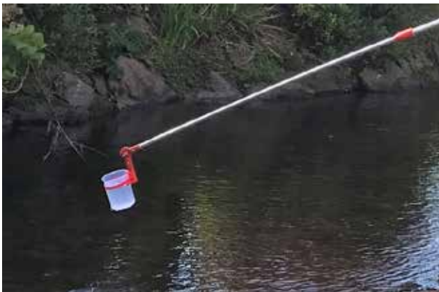
Figure 6.4 A scoop on an extendable pole used for taking surface samples © Deborah Chapman
