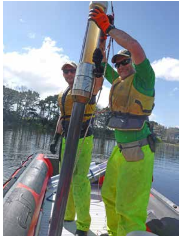
Figure 6.11 Removing an intact sediment core from Lake Nganoke, New Zealand. By Susie Wood Lakes380, Licenced by CC BY-SA 4.0, via Wikimedia Commons
