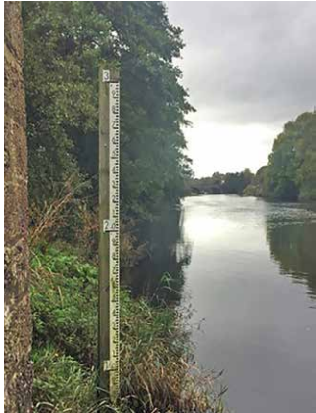
Figure 2.8 A simple staff gauge for measuring water level © Patrick Cross
