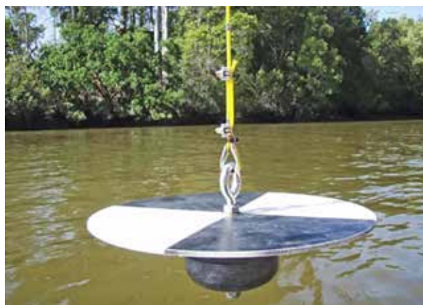
Figure 6.16 A secchi disc for measuring the transparency of the water (DES 2018) By State of Queensland, Licenced under CC BY 3.0 AU
