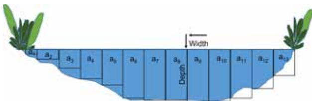
Figure A.1 Dividing a cross section of a river into equal width vertical columns in order to calculate cross-sectional area
