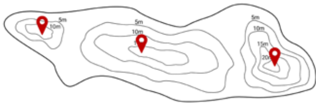
Figure 6.18 Example of a bathymetric map showing a lake with three sub-basins and the potential locations of three sampling stations
