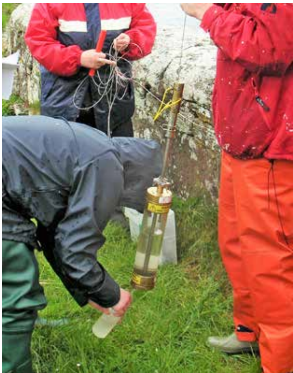
Figure 6.5 Emptying a depth sample from a Ruttner sampler into sample bottles © Deborah Chapman
