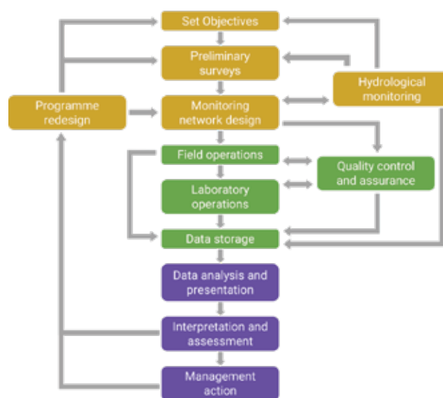
Figure 1.1 The chain of activities in designing and implementing a freshwater quality monitoring programme (adapted from Chapman, Meybeck and Peters 2005)
