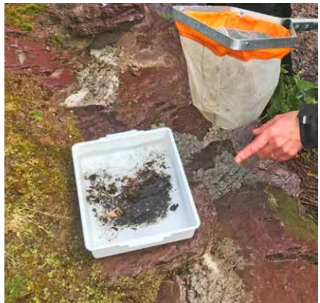
Figure 6.9 A D-net used for collecting a macroinvertebrate sample that has been emptied into a white tray for sorting and identification © Deborah Chapman
