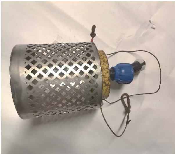
Figure 18: Use of a steel basket for prevention of clogging the sampling device (© IWRS, 2022).
