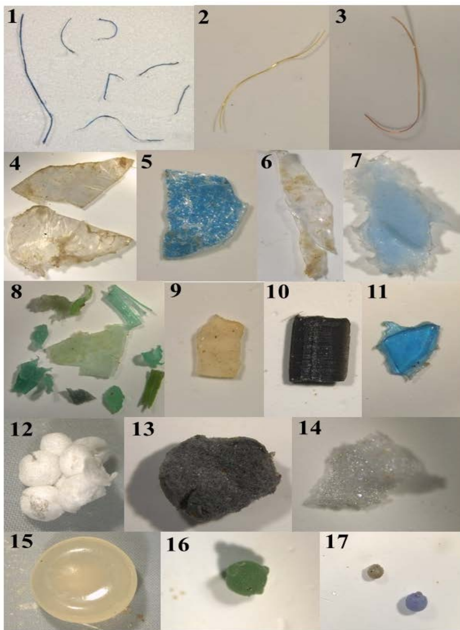
Figure 11: Common shapes of microplastics. (1: fibers, 2-3: filaments, 4-7: films, 8-11: fragments, 12-14: foams, 15: pellet, 16-17: granule) (Photo: © Ülgen Aytan, Turkey).
