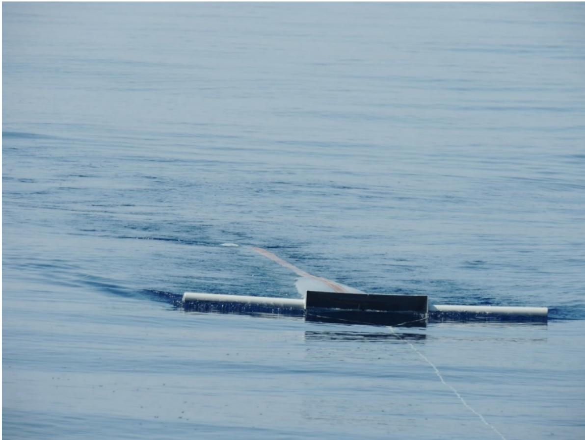
Figure 7: Manta net being operated in calm sea, outside of the bow wave caused by the spinning of the propeller (Photo: © Christos Ioakeimidis, UNEP/MAP).
