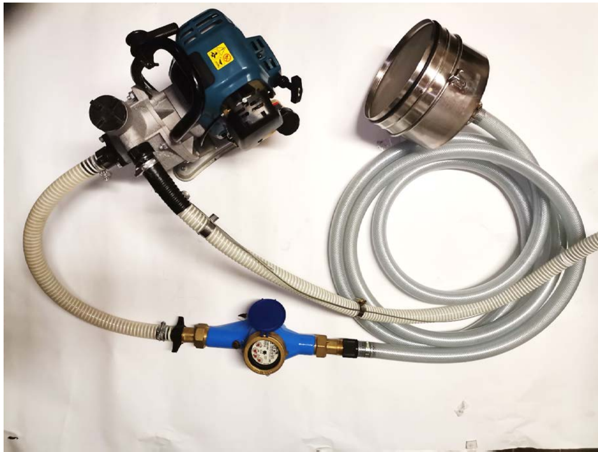
Figure 26: A small and light weight water pump with a mounted flow meter (© IWRS, 2022).
