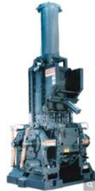
Figure 2.8: The Banbury mixer, used for the mixing of polymers and additives in the manufacture of plastic and rubber. Courtesy of Farrel Corporation
