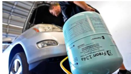
Refrigerants used in fridges, freezers and cars change from a fluid to a gas to transport heat away from the place you want cooled.
