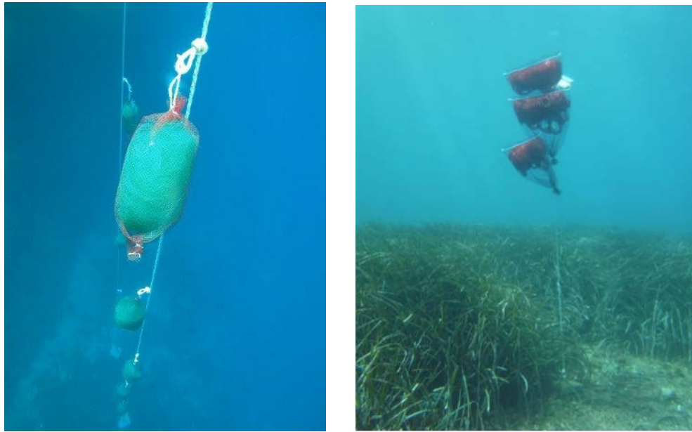
Fig. 3. Larval collector bags attached in 1,5 m intervals in a deep site (left) and a shallow site installation (rightly). Photographs: D. K. Kersting, I. E. Hendriks.
