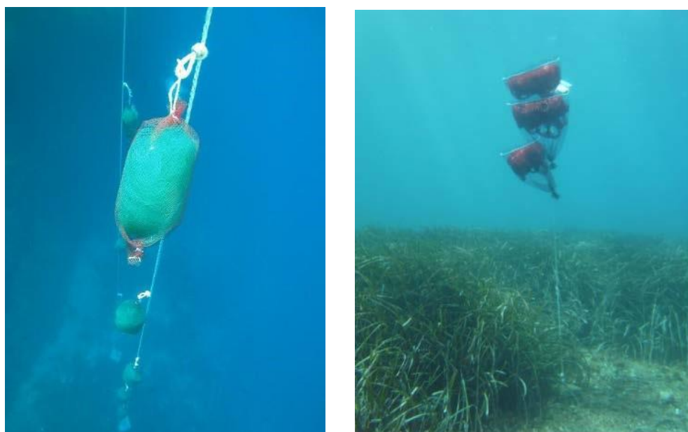
Fig. 3. Larval collector bags attached in 1,5 m intervals in a deep site (left) and a shallow site installation (right). Photographs: D. K. Kersting, I. E. Hendriks.
