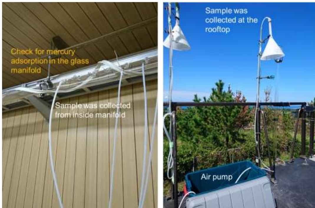
Fig. 2 Photo of the test measurements during September 21-22, 2021. The left one shows sampling through manifold, and the right one shows sampling without manifold.
