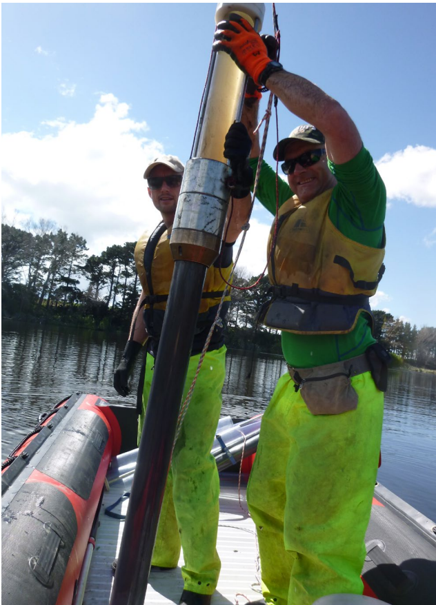
Figure 5.5 Removing an intact sediment core from Lake Nganoke, New Zealand. By Susie Wood Lakes380, Licenced by CC BY-SA 4.0, via Wikimedia Commons
