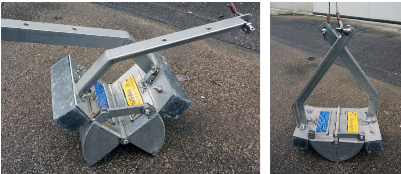
Figure 5.4 A Van Veen benthic grab sampler with jaws open (left) and closed (right). © Patrick Cross
