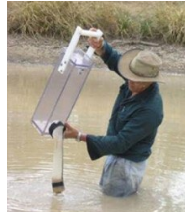
Figure 5.9 Collecting a quantitative zooplankton sample with a Schindler-Patalas trap (Department of Environment and Science 2018) By State of Queensland, Licenced under CC BY 3.0 AU
