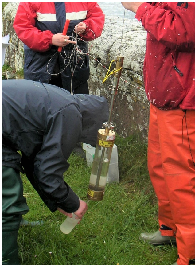
Figure 5.6 A bottle sampler that can be lowered to a required depth before being triggered to close by a heavy messenger that travels down the suspension cable. The bottle is brought to the surface to be emptied. © Deborah Chapman
