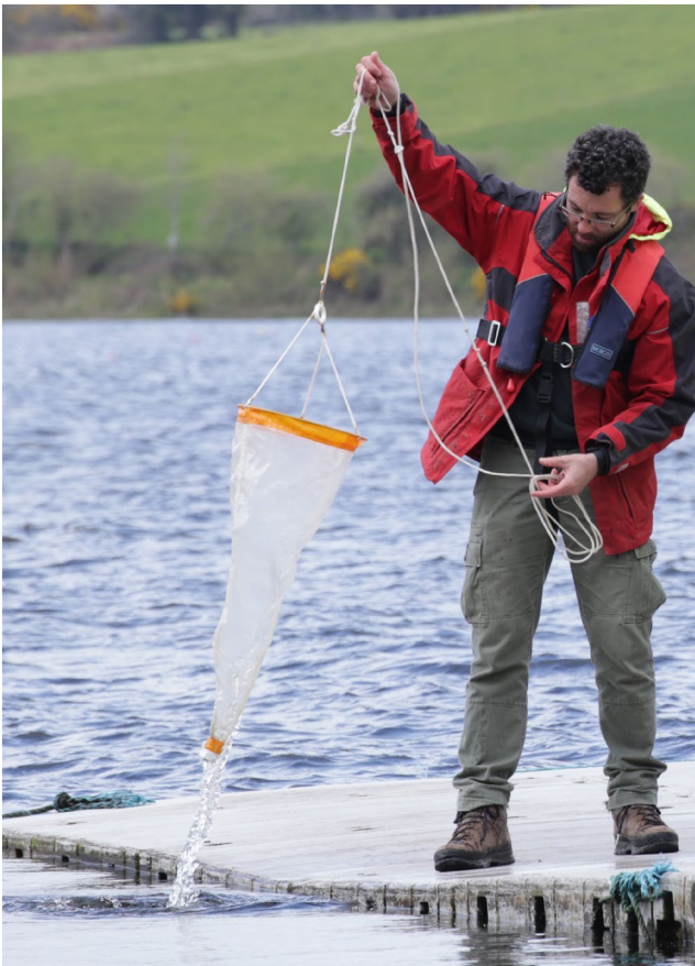
Figure 5.8 Collecting a qualitative plankton sample by drawing a plankton net through the water column of a reservoir. © Patrick Cross
