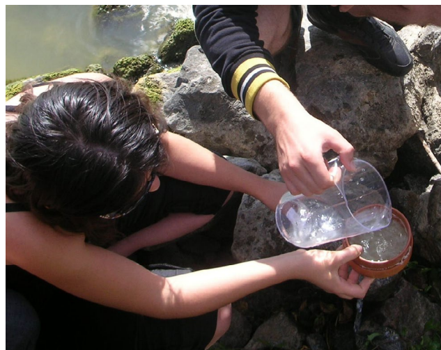
Figure 5.7 Obtaining a quantitative plankton sample by filtering a measured volume of water through a filter cup with a plankton mesh of known pore size. © Deborah Chapman
