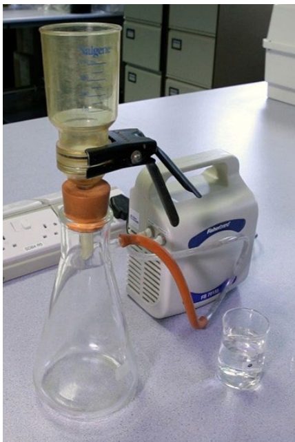
Figure 4.1 A simple filtration apparatus that can be used for filtering bacteria from measured water samples. © Patrick Cross
