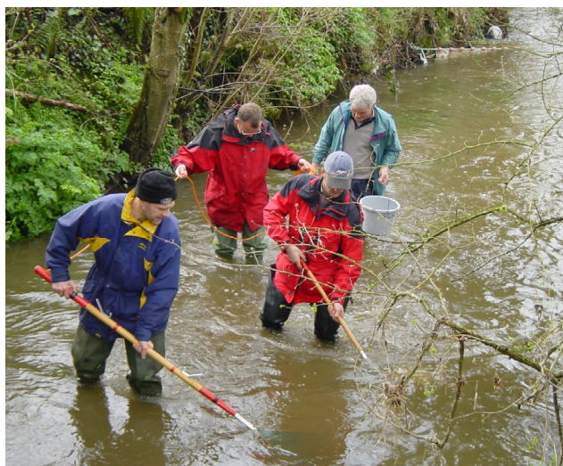
Figure 5.11 Electro-fishing is a non-destructive method for obtaining a quantitative estimate of fish populations. © Deborah Chapman
