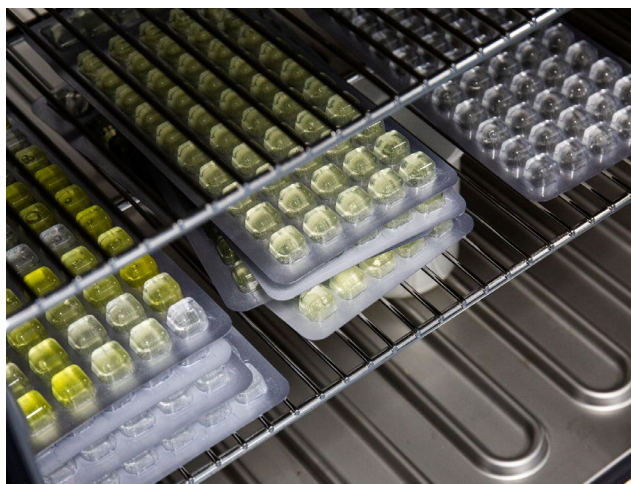
Figure 4.3 Multiple-well trays in an incubator. Each tray contains a 100 ml sample mixed with an enzyme substrate to enumerate total coliforms and E. coli . © Environmental Research Institute (ERI), UCC
