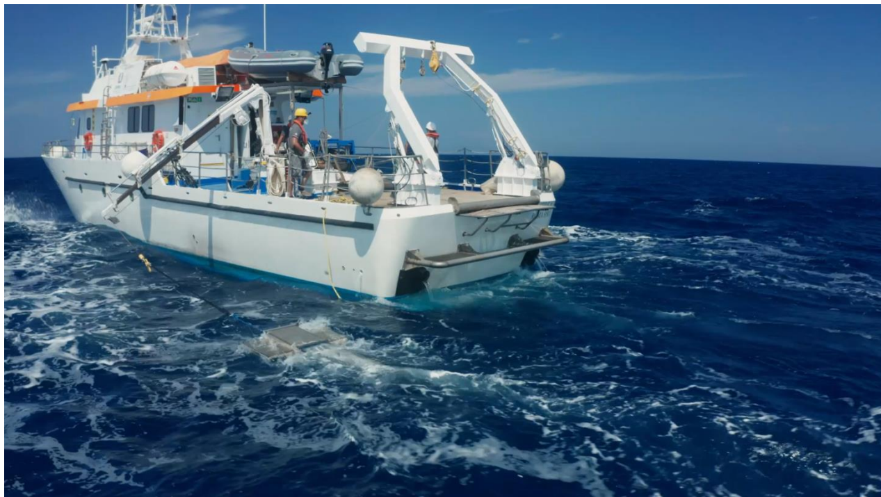
Figure 9: A manta net being pulled from the side of the vessel (Credit © Cecilia Silvestri & Marco Matiddi, Italy)
