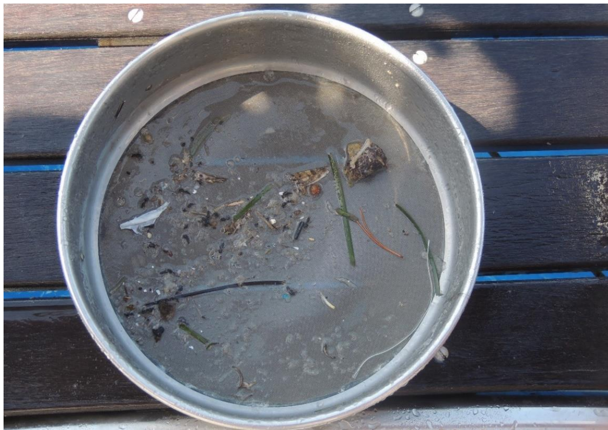
Figure 10: Microplastic and organic matter collected in a metal sieve just after the sampling (Photo: © Christos Ioakeimidis, UNEP/MAP).
