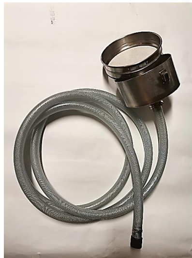
Figure 193: A PVC hose with a filter system with a stainless-steel sieve (100 µm) (© IWRS, 2022).
