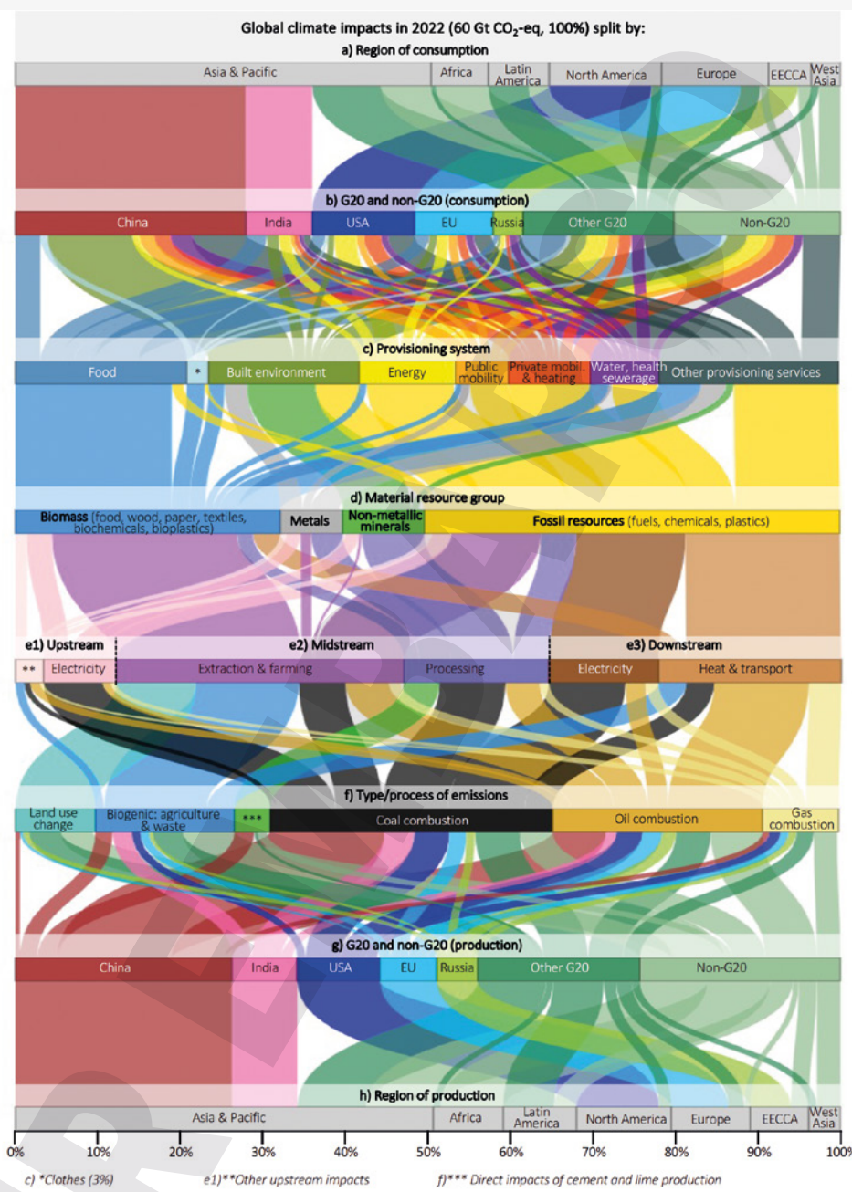
Figure 3.16: Supply chain mapping of global climate impacts in 2022 (total 55 Gt CO 2 -equivalents, 100%). Each bar adds up to 100% and shows the global climate impacts from different perspectives in the global supply chain such as
