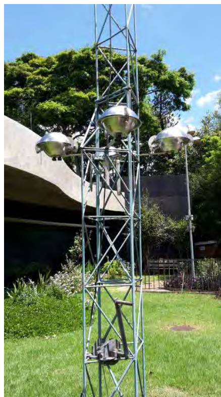
Sampling site for air with PAS/PUF: Brazil, © Environmental Company of the San Pablo State
