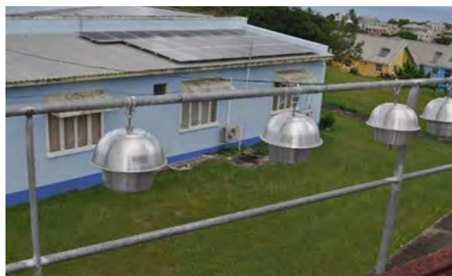
Sampling site for air with PAS/PUF: Barbados, © Ministry of Environment and Natural Beautification
