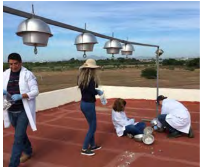
Sampling site for air with PAS/PUF: Mexico, © National Institute of Ecology and Climate Change (INECC)
