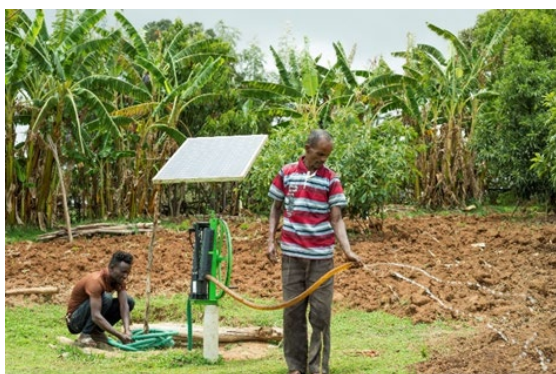
Using a solar-powered water pump to pump groundwater for irrigation in Ethiopia (Maheder Haileselassie / IWMI)
