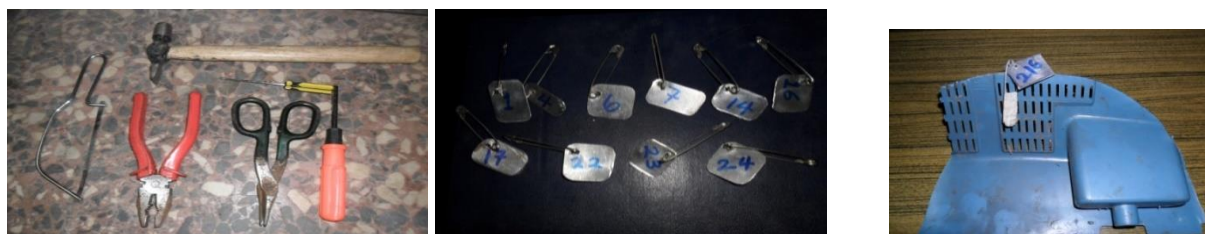
Figure 7: Sampling tools for cutting WEEE plastic, labelled tags and CRT plastic casing with tag
