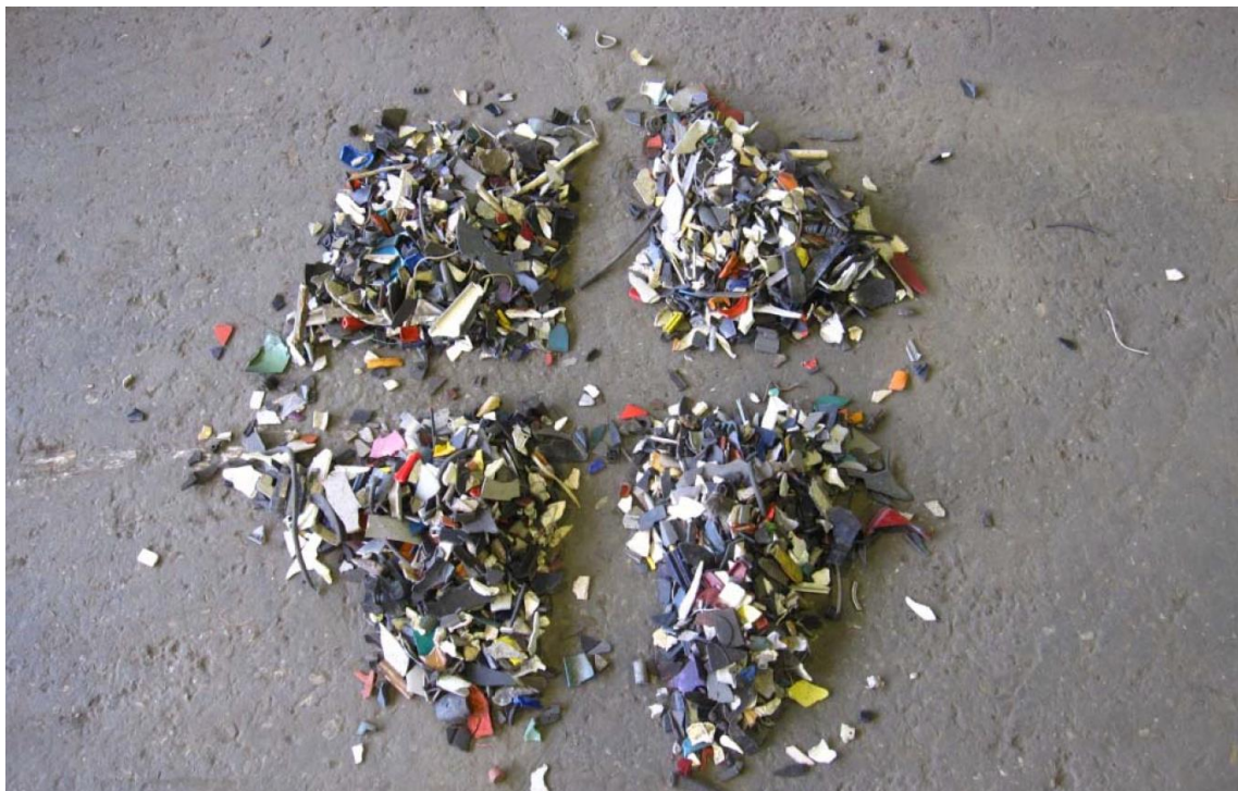
Figure 11: Flat heap of WEEE plastic separated in quarters by two diagonals for reducing sample volume
