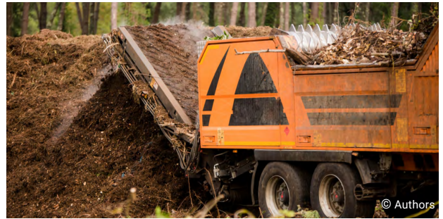
Figure 11: A shredder breaking up woody waste
