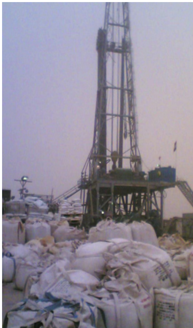
PHOTO 6: Poor storage of chemicals
